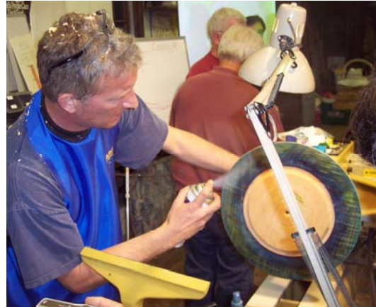
.Jimmy sprays a mixture of alcohol and 5% shellac on the rim of the platter to seal the color.
