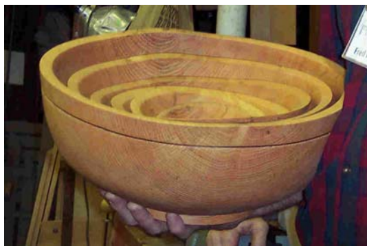
Fred Ayers nest of Red Oak bowls turned and cored with a One Way coring system.
